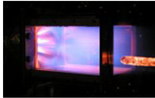
Combustion experiments with model combustor (On the right is a probe for gas-analysis)
